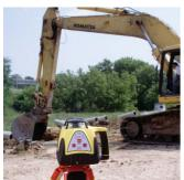
The RUGBY 100LR is an automatic self-leveling general construction laser for exterior jobs of any size, large or small. You can use it for:
