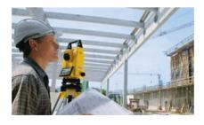
The Builder R100M and R200M with built-in memory, saves and transfers measured data via an interface between the Builder and a PC.
