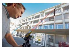
Indirect height-measurement: Window heights can be determined using the Pythagoras function.
